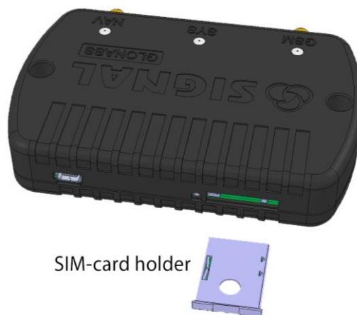
Figure 22. SIM-card installation to the device
