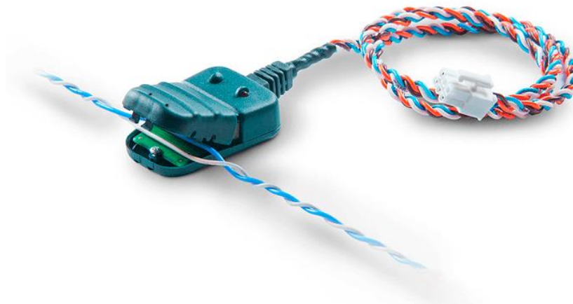
Figure 48. Connection to CAN through contactless reader
