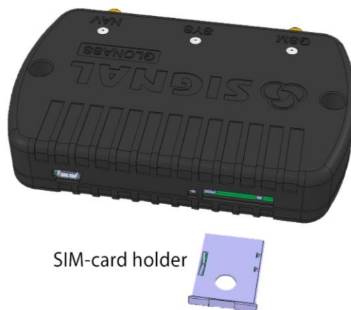
Figure 22. SIM-card installation to the device
