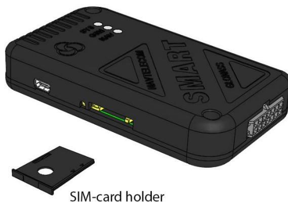
Figure 17. SIM-card installation to the device
