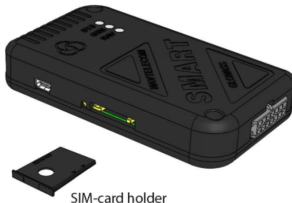
Figure 17. SIM-card installation to the device
