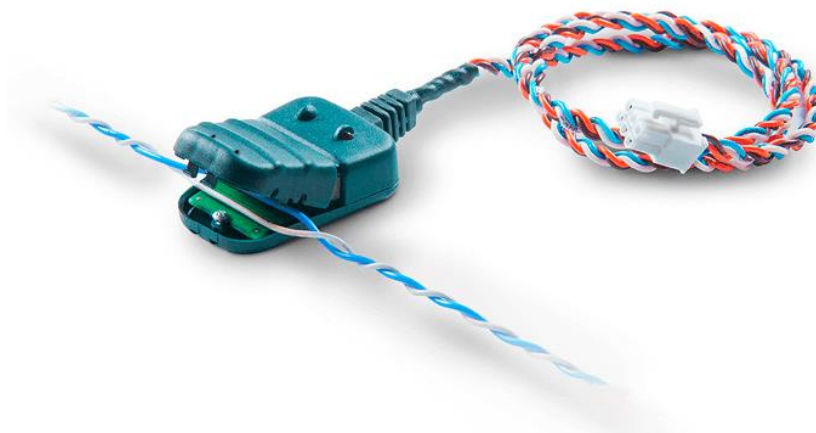
Figure 42. Connection to CAN through contactless reader
