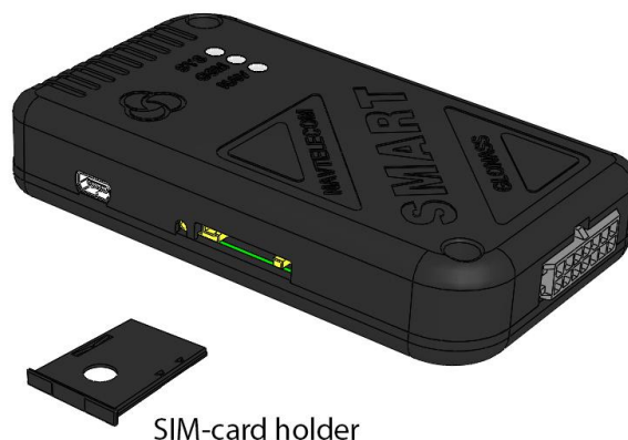
Figure 18. SIM-card installation to the device
